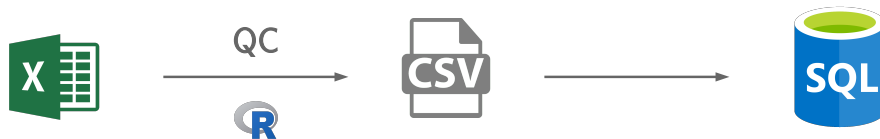
Figure 5. STAR import procedure, showing the flow of data from the Excel template, import into R, export to CSV format, and import into the database. The R import step runs a suite of QC tests to check for common errors.
